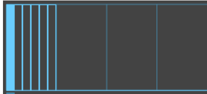
waveform = square, level = 1.0, pulse width = 0.25
